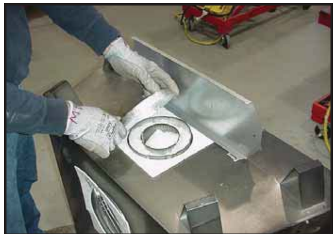
Figure 7.4 Remove the vent cap.
