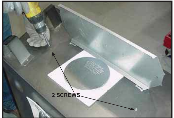
Figure 7.3 Replace the two screws as shown.
