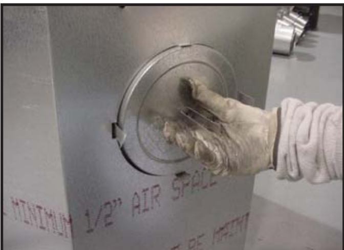
Figure 7.8 Fold the center parts of the retaining band out and use to remove the vent cap.
