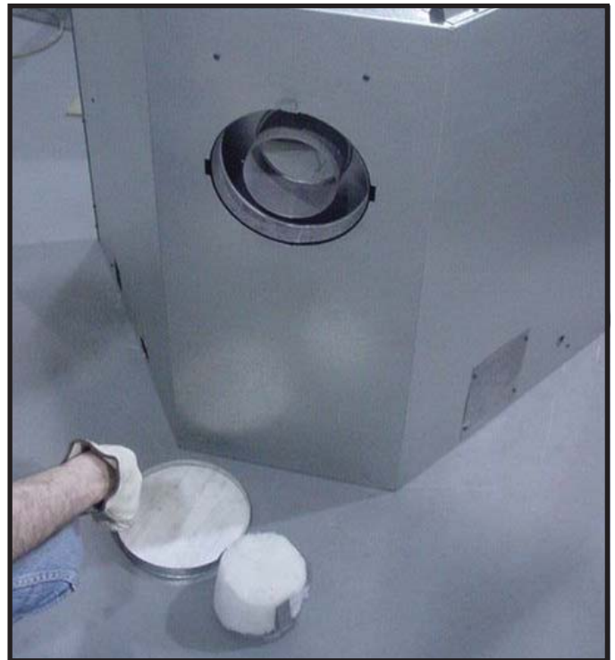
Figure 7.9 Discard the vent cap, remove and discard the insulation basket. Note: Once the vent cap has been removed it CANNOT be reattached.
