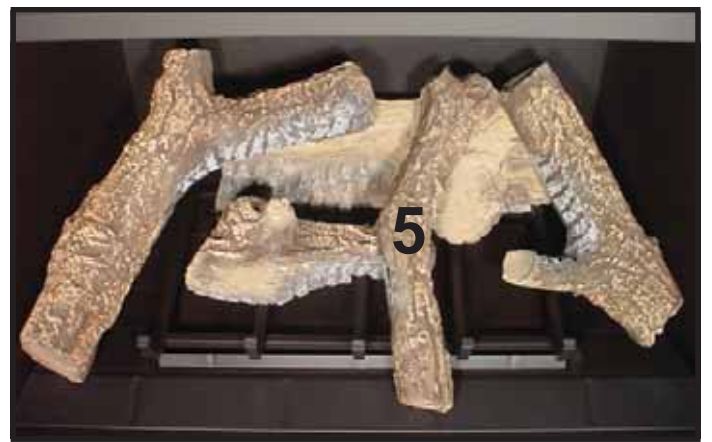
LOG #5 (SRV385-723): Position log #5 between the 3rd and 4th grate bar resting on the grooves in log #1 and log #2.
