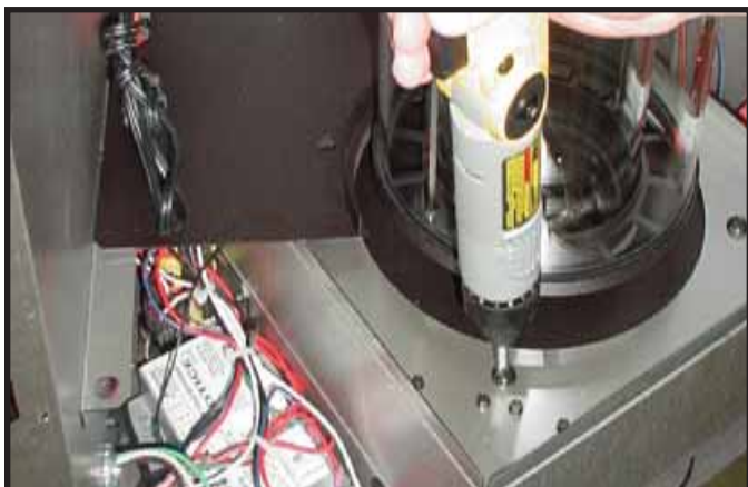
Figure 12.6 Continue until all four screws have been bottomed out and the glass cylinder is in place. Reverse these steps to remove the assembly.
