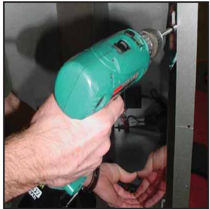
Figure 14.1 Using a 1/4 inch nut driver remove the reflector panels as shown.
