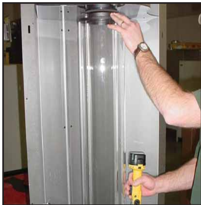
Figure 12.5 Hold the top of the assembly back against the stops while raising the platform as shown.
