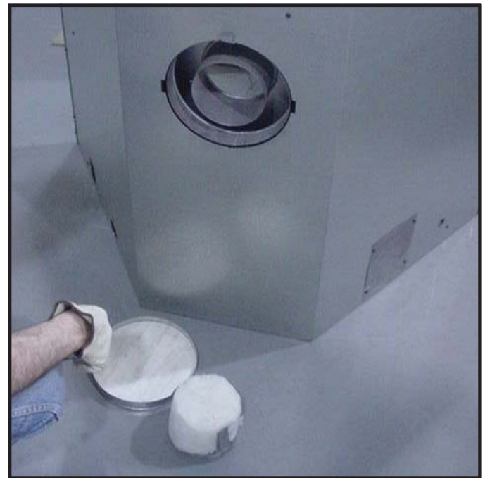
Figure 7.9 Discard the vent cap, remove and discard the insulation basket. Note: Once the vent cap has been removed it CANNOT be reattached.
