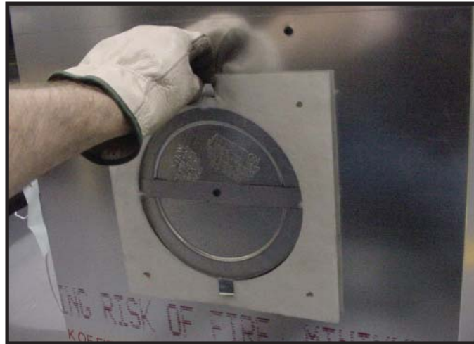
Figure 7.6 Fold the tabs toward the center of the fire plug (90°) and remove the insulation gasket.
