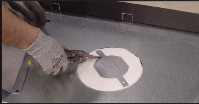
Figure 7.2 Cut the seal cap strap across the rectangles next to the disk. The top heat shield may need to be removed to perform this step.
