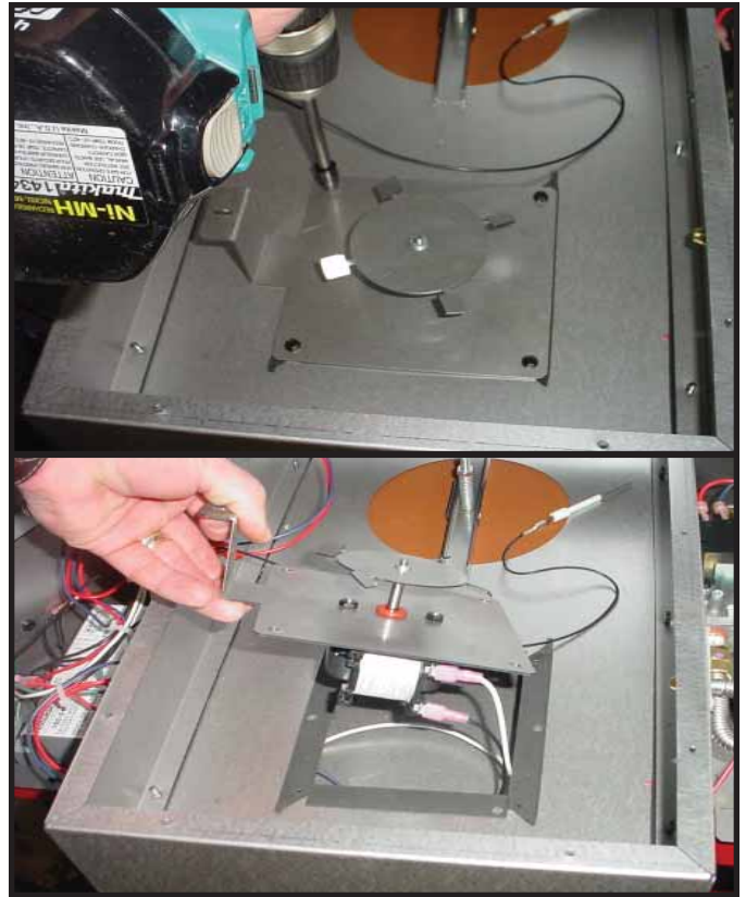
Figure 14.4 The fan plate can now be accessed. Remove the four screws. Lift the fan plate, being careful to not cut or scar wiring while disconnecting them from the fan motor.
