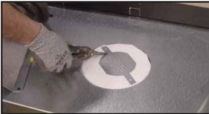
Figure 7.2 Cut the seal cap strap across the rectangles next to the disk. The top heat shield may need to be removed to perform this step.
