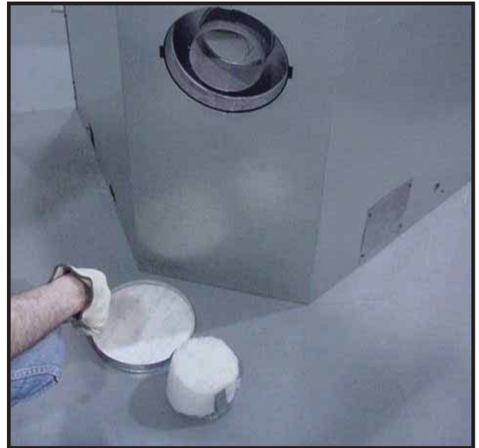
Figure 7.9 Discard the vent cap, remove and discard the insulation basket. Note: Once the vent cap has been removed it CANNOT be reattached.
