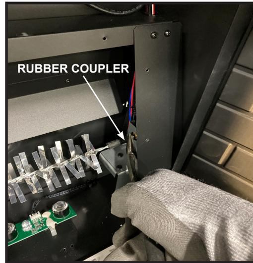
Figure 12 Rotisserie Rod Removal
