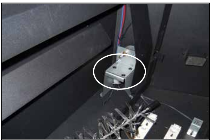
Figure 17 Location of three Screws that attach Motor Mount Bracket to Appliance
