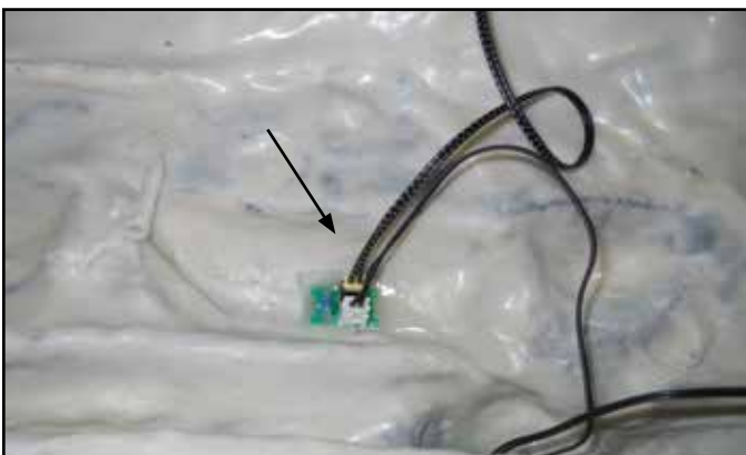
Figure 3 Light LED Connection on Bottom of Log Ember Bed
