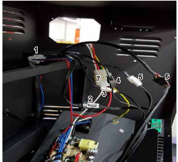
Figure 10 Seven Electrical Connections required for Heater/ Blower Module Removal and Installation
