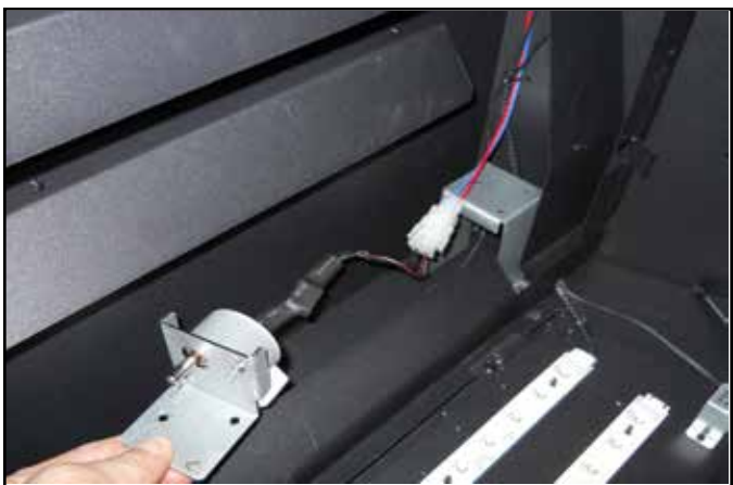
Figure 18 Electrical Connection required for replacement for the Faux Flame Motor.
