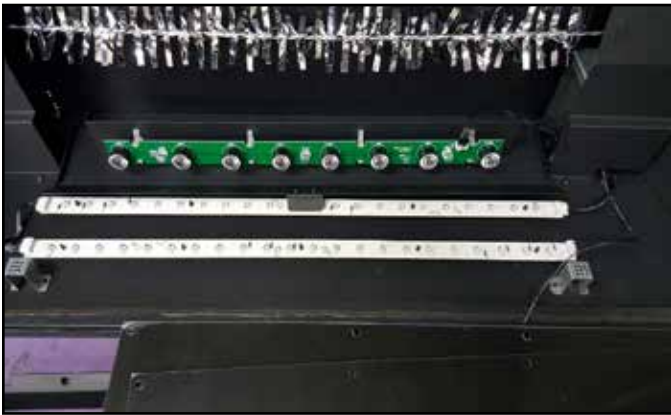
Figure 7 Light LED Circuit Power Source Connectors for 36\"/>
