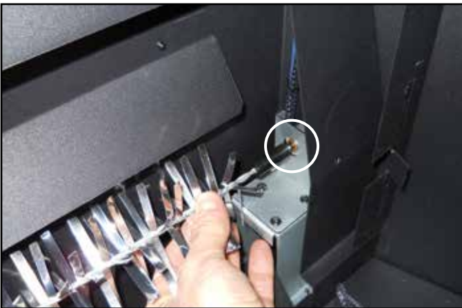
Figure 15 Removal and Installation of Reflector Rod Coupler to Motor Shaft
