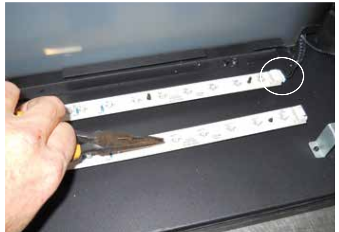
Figure 5 Barbed Clip Access during LED Circuit Board Replacement
