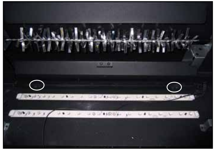
Figure 4 Removal and installation of 30" LED access panel
