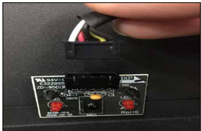
Figure 12 Disconnect Wiring Harness from Remote Receiver Board
