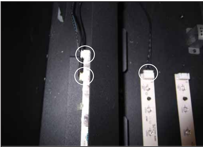
Figure 6 Light LED Circuit Power Source Connectors
