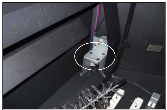
Figure 16 Location of three Screws that attach Motor Mount Bracket to Appliance
