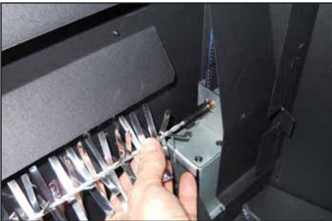
Figure 14 Removal and Installation of Reflector Rod Coupler to Motor Shaft
