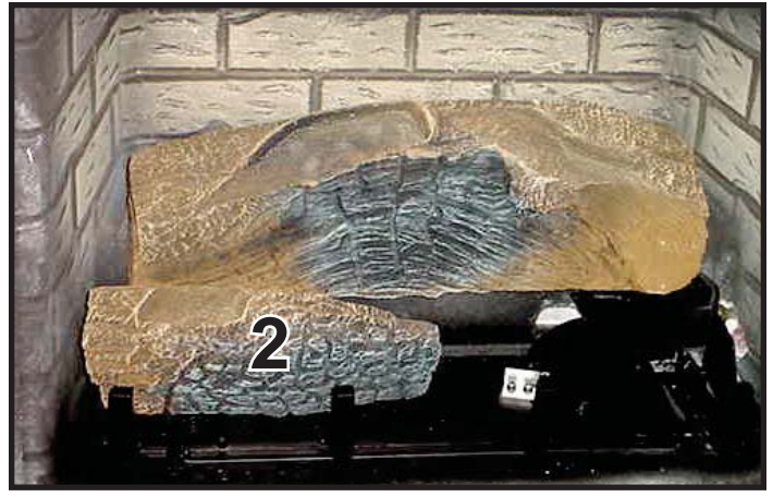
LOG #2 (SRV2019-702): Position log #2 by locating its slot over the tabs on left front of the burner.
