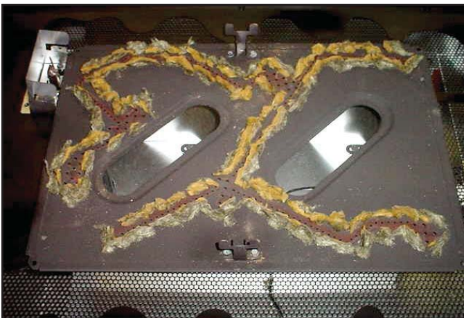
Figure 42 Placement of the Ember Material
