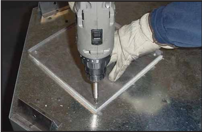
Figure 7.1 Remove the cover plate by removing the four screws holding it to the top of the appliance. Remove and discard the cover plate.
