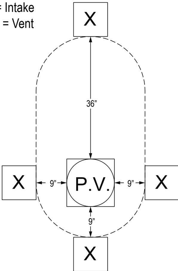
Minimum Clearance Using an RS Series Powervent
