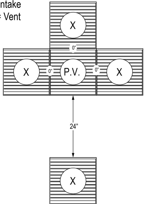
Minimum Clearance Using an In-Line Powervent
