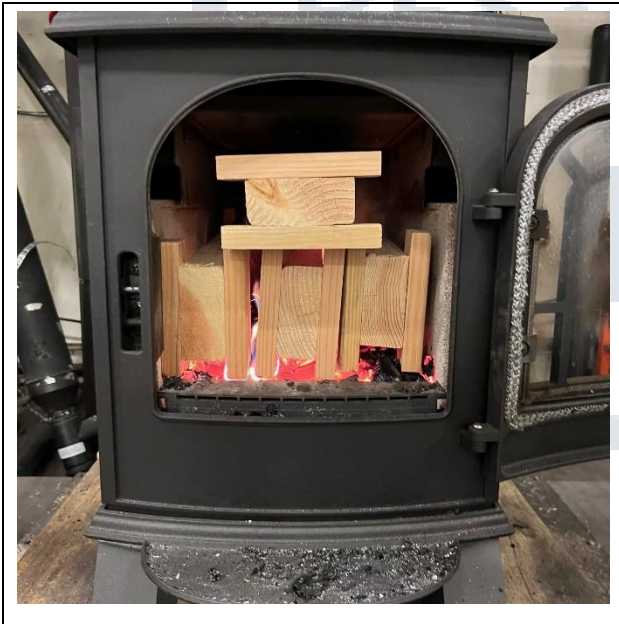
Test Fuel Loaded in Stove
