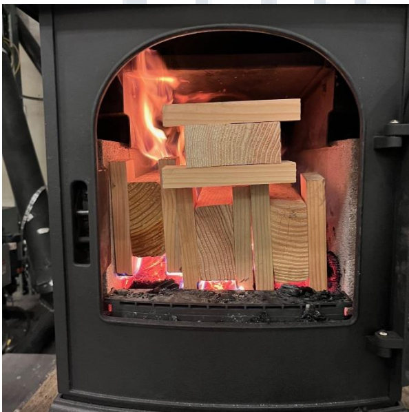
Test Fuel Loaded in Stove
