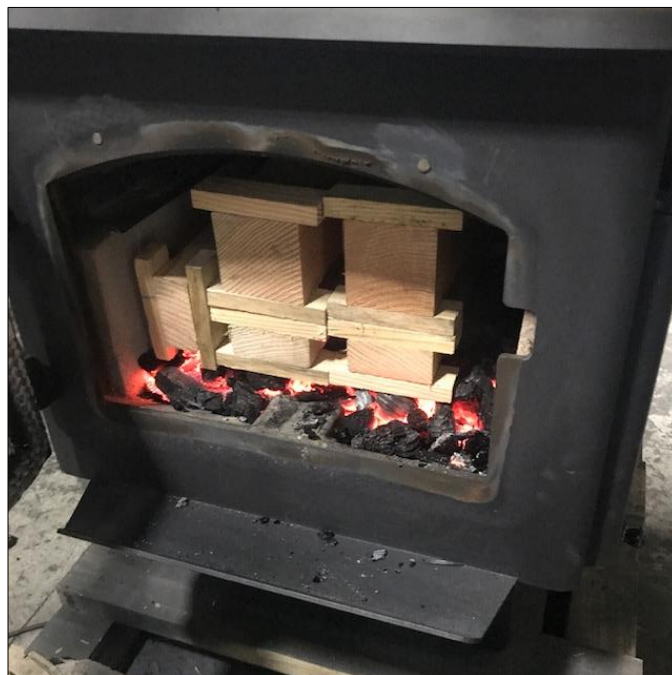
Typical Test Fuel Loaded in Test Stove
