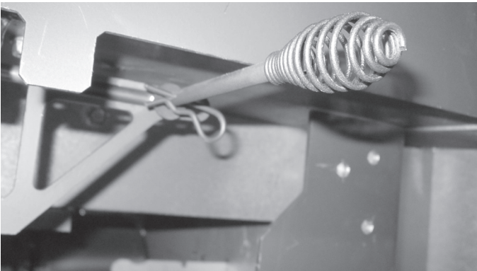
Figure 4.25 Reinstalling Hairpin Clip and Washer
