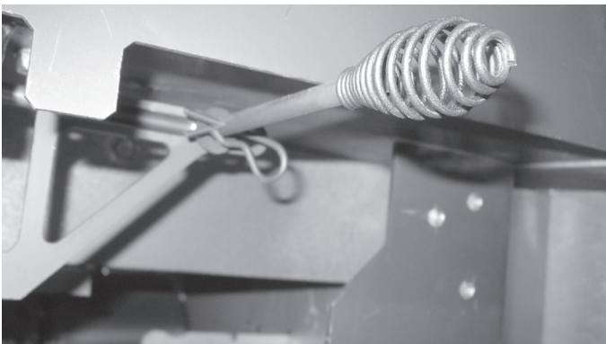
Figure 4.25 Reinstalling Hairpin Clip and Washer
