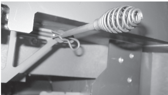
Figure 4.36 Reinstalling Hairpin Clip and Washer
