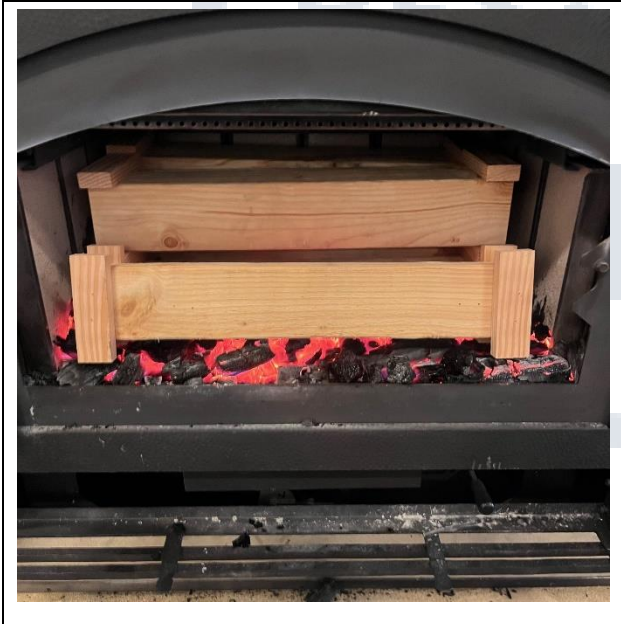
Test Fuel Loaded in Stove
