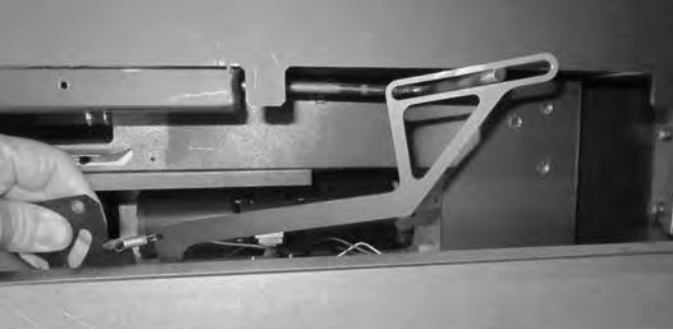
Figure 4.23 Inserting Timer Assembly
