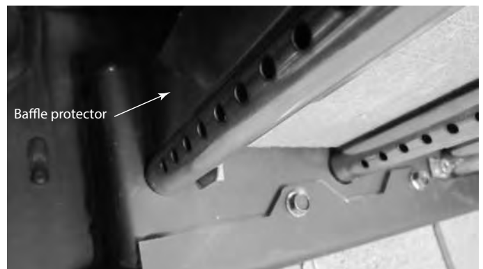
Figure 4.9 Reinstall Baffle Protection Channel
