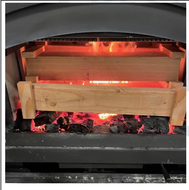
Test Fuel Loaded in Stove
