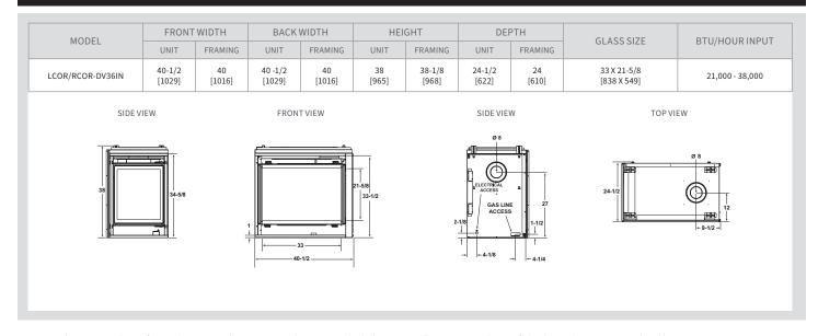
Dimensions shown are in inches. Reference dimensions only. We recommend measuring individual units at installation. Assumes the use of 1/2" Sheetrock. NOTE: Non-combustible material is allowed over this dimension. Make sure you do NOT cover the decorative door opening.
