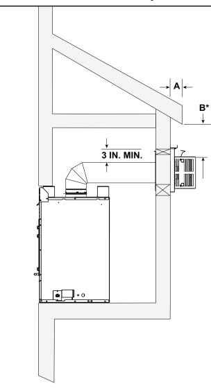
\* NOTE: If overhang (A) is less than 2 inches, clearance from top of termination cap to bottom of overhang (B) may be 0 inches.
