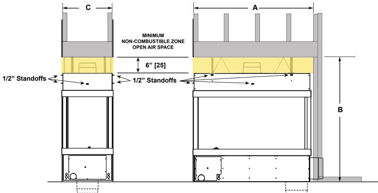
**NOTE: Fireplace MUST be square in both directions prior to finishing or the glass will not fit properly.**
