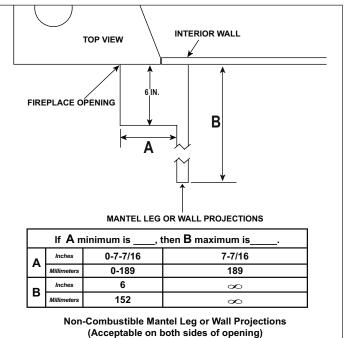
If using heat management please refer to the fireplace installation manual for framing guidelines and reduced mantel clearances. Additional information on venting, TV clearances, finishing requirements, fronts, etc can be found in the installation and owner's manual
