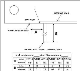
Combustible Mantel Leg or Wall Projections (Acceptable on both sides of opening)
