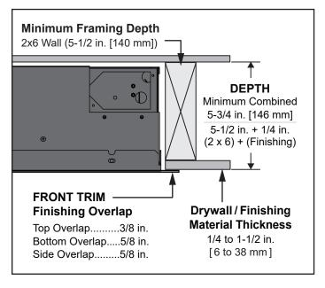
The Allusion Edge slides into a framed and finished wall and is compatible with finishing materials such as painted drywall, tile, and other smooth finishes such as porcelain and granite.
