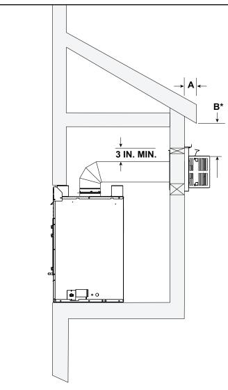
\* NOTE: If overhang (A) is less than 2 inches, clearance from top of termination cap to bottom of overhang (B) may be 0 inches.
