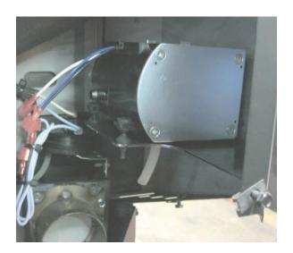
**Step 9.** Attach the light blue and the yellow wires from the pump to their color corresponding wires from the harness. Neatly tie all of the wiring away from any moving parts and rub points. Stay clear of the pusher arm and the heat from the igniter element.
