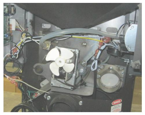
**Step 11.** Test operation; with the igniter switch in the auto position, and the Feed Adjuster on #2 or #3, turn the mode selector to STOVE TEMP and the temperature dial to #7. Listen for the air pump to run. If you do not hear it running, turn to "OFF" immediately, to protect the igniter from damage.
