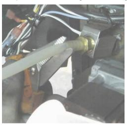
**Step 3.** Carefully cut the wire ties from the bundle of wires. DO NOT CUT INTO THE WIRES. Disconnect the power wires from the harness to the air pump. Follow the ground wire from the pump to the mounting point on the feeder heat shield. Cut and discard the ground wire, it will not be needed.
