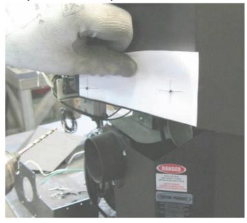
**Step 6.** Be sure the large round hole in the mounting bracket is open. If it is not, simply break it away. Hold the mounting bracket in place inside the rear cabinet. Proper positioning is with the pointed end of the bracket toward the back and the long bent tab (pointing downward) going in toward the front of the stove. Align the two holes in the bracket with the two holes you just drilled, and secure using two black pop-rivets.
