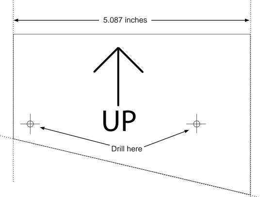
Template; Cut or fold on the dotted lines. Edges or folds will fit the bends of the hopper sheet metal.
