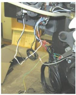
**Step 4.** Using a 3/32 Hex Key Wrench, remove the existing pump mounting screws. Begin by removing the two bottom screws, then support the pump as you remove the top two screws. You will not be re-using these screws. This picture shows what you should be seeing with the pump removed and disconnected.
