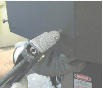
**Step 7.** Using a minimum 3 inch extension, install the 5/16" driver-bit into your drill or screw-gun. To level the mounting bracket, align the bottom of the bent tab on the bracket with the bottom of the hopper sheet metal. Using the two holes in the mounting bracket tab, install two self drilling Tek screws into the hopper sheet metal to secure the front of the mounting bracket.
