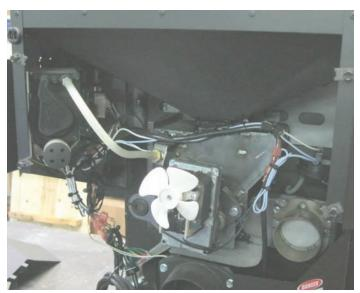
**Step 2.** Remove or cut the 1/4" silicone tubing from the existing air pump. At the igniter end, cut the tubing even with the end of the igniter fitting, leaving a short piece of 1/4" tubing on the fitting.
