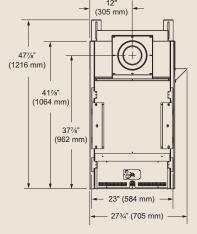
Framing dimensions in illustrations accommodate 1/2" finishing material.
