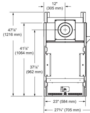
Framing dimensions in illustrations accommodate 1/2" finishing material.
