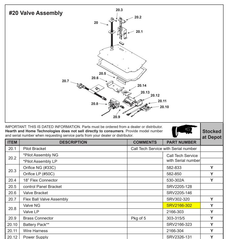
SRV046-018A 20.14 Thermostat Assembly \*\*Fuse for battery pack can be sourced locally, not a warranty item. Specs are 250v, 1A fuse, 3/4" long
