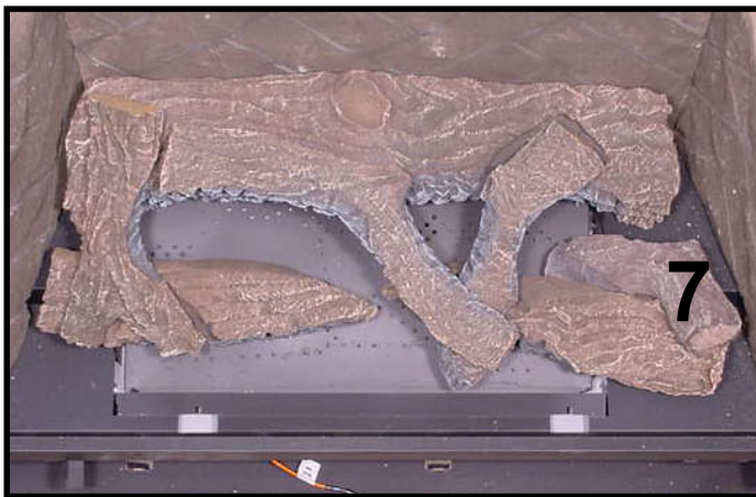
LOG #7 (SRV740-707): Small log #7 rests on the “ramp” on the backside of log #3. The burned out end of the log slopes down and to the left.
