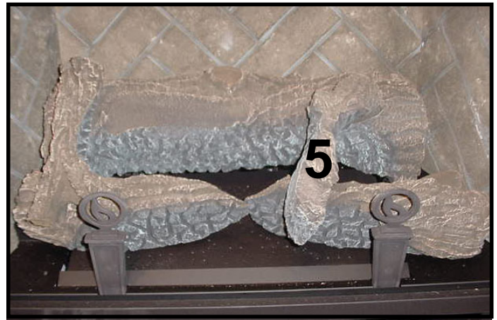
LOG #5 (SRV340-706): Place log #5 across log #1 and log #3. The notch in the bottom of the log sets on the carved out edge on top of log #3. The back of the log sits in the grooved out area in log #1.
