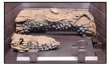
LOG #2 (SRV310-702): Position log #2 by locating its slot over the tab on the front left of the burner. The slot in the left end of the log slides into the metal edge in front of the square cut out on the base pan.
