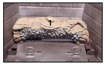
LOG #1 (SRV310-701): Place log #1 in the back on the insert. Locate the legs of the log to either side of the burner. Pull the log forward until the log is stopped by the back edge of the burner. Slide the log to the left so it touches the left wall of the fireplace.
