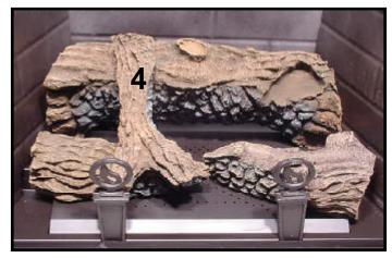
**LOG #4 (SRV340-704):** Nest log #4 in the smooth cut-out areas on the left side of log #1 and right side of log #2. The "Y" end of log #4 rests on log #2.
