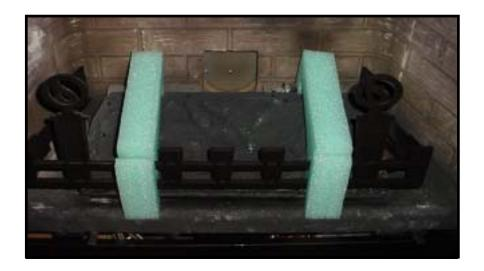
Place grate on the base of the firebox surrounding the burner. The grate should be centered on the burner and pushed back until it contacts the burner.
