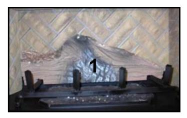
**STEP 2:** LOG #1 (SRV2016-701): Place notches of log #1 on outer two grate tines, and push against back of firebox.
