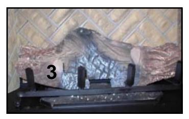
**STEP 4:** LOG#3 (SRV2014-703): (This log is the same as log #2). Place log #3 with the flat side down and burned side into notch on burner. Pull left end forward against grate.
