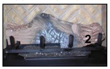
**STEP 3:** LOG #2 (SRV2014-703): Place log #2 with the left tip of the log on the flat spot on the burner. Pull the right part of the log to touch right grate tine, and the top of the log should rest against log #1.
