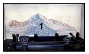
**STEP 2.** Place log #1 (SRV2016-701) centered on grate and 1 inch from back of firebox.
