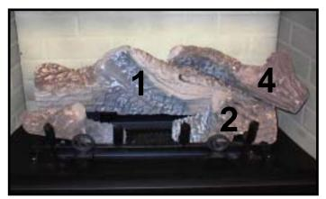
**STEP 5.** Place log #4 (SRV780-707) across log #1 and log #2 with left end touching the back of the firebox, and the right end overhanging log #2 by 3 inches.
