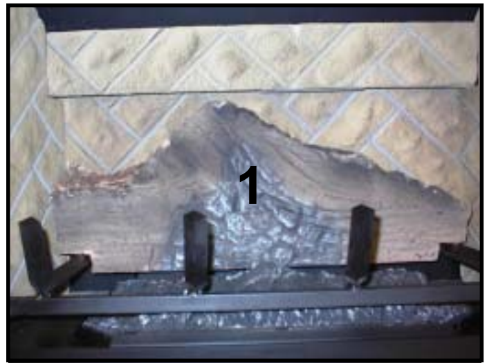
STEP 2: LOG #1 (SRV2014-701): Place log # 1 centered on the grate and pushed against the back of firebox.
