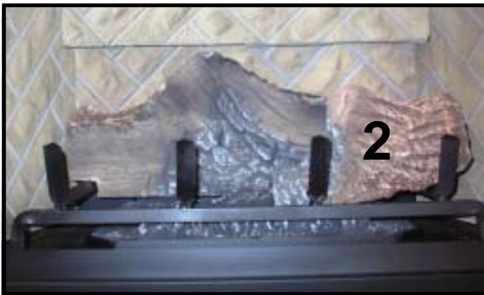
STEP 3: LOG #2 (SRV2014-703): Place log # 2 with the left tip of the log on the flat spot on the burner and the right end pulled forward against grate.
