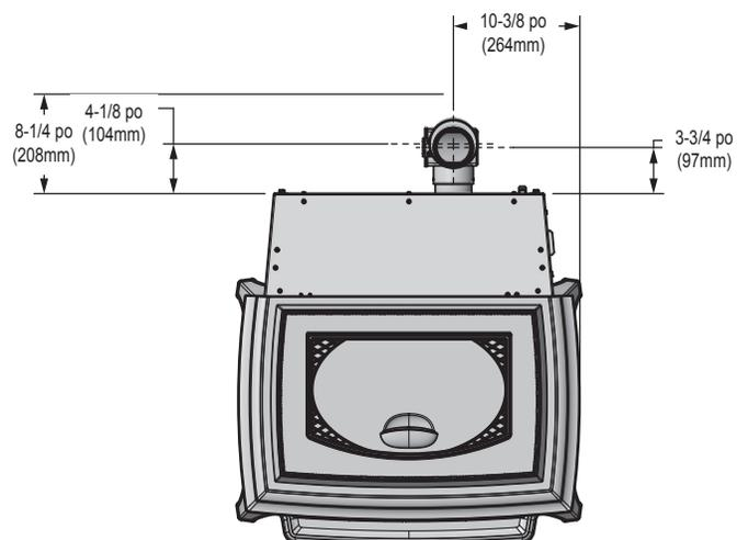
Figure 7.4 - Top View with Top Vent Adapter (TPVNT-6) and Offset Adapter (811-0720).
