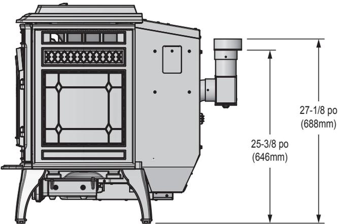
Figure 9.1 - Side View with Top Vent Adapter (TPVNT-6) and Offset Adapter (811-0720).
