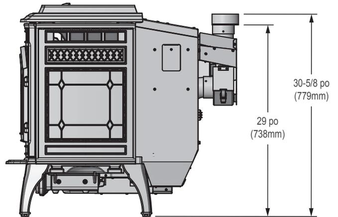
Figure 8.3 - Side View with Top Vent Adapter (TPVNT-3) and Offset Adapter (811-0720).
