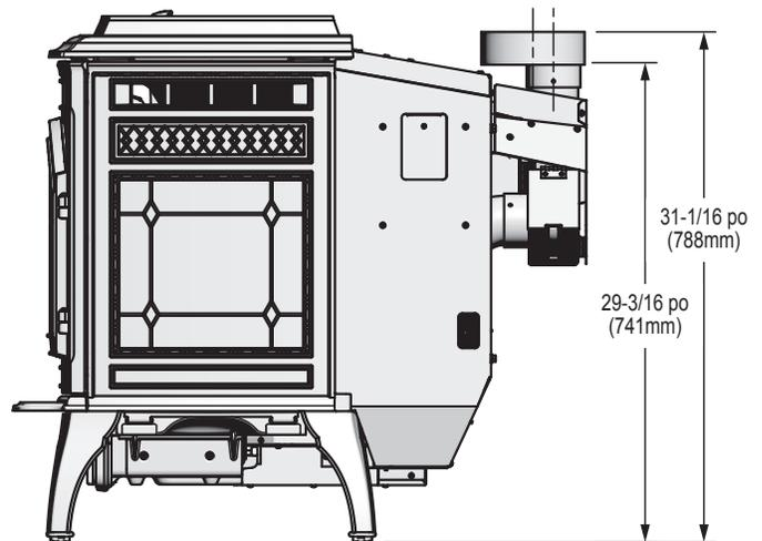
Figure 8.4 - Side View with Top Vent Adapter (TPVNT-3) and Offset Adapter (812-3570).
