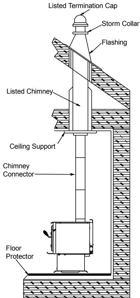
Figure 18.1 - Prefabricated Interior Chimney
