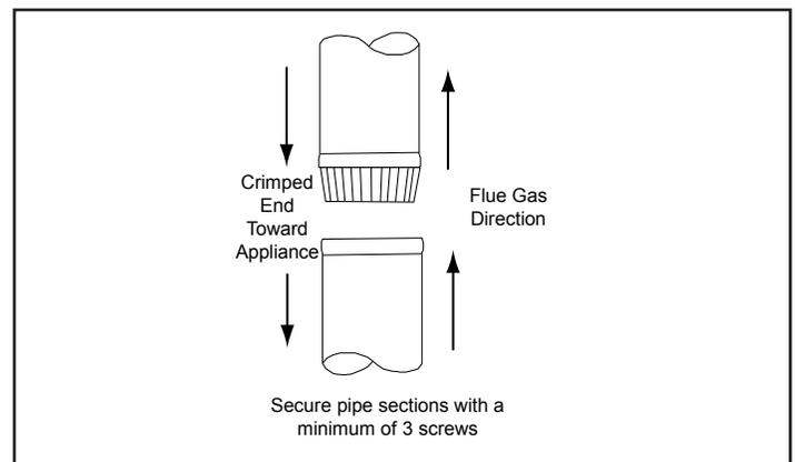
Figure 19.3 Chimney Connector (Appliance Pipe)
