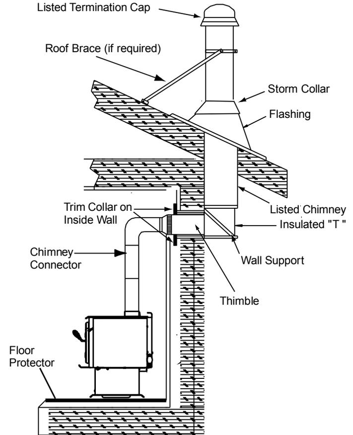
Figure 17.1 Prefabricated Exterior Chimney
