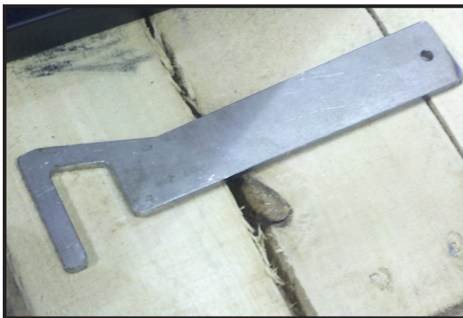
Figure 11.1. Glass Clip Tool
