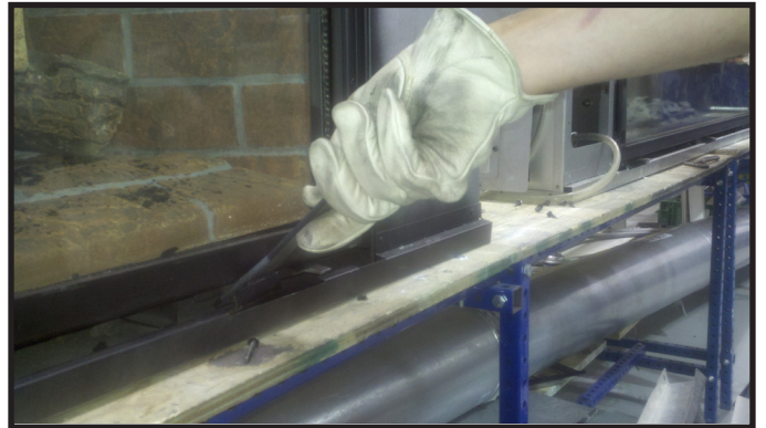
Figure 11.3. Inserting Glass Clip Tool
