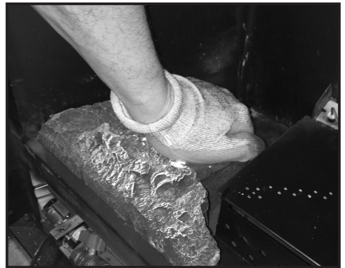
Figure 11.2 Press Left Hearth Firmly Into Place
