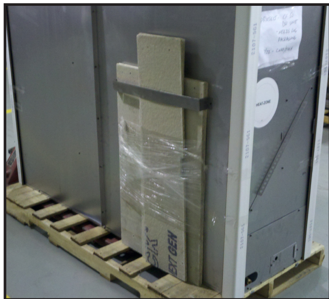
Figure 6.6 Shipping Location of Non-Combustible Board
