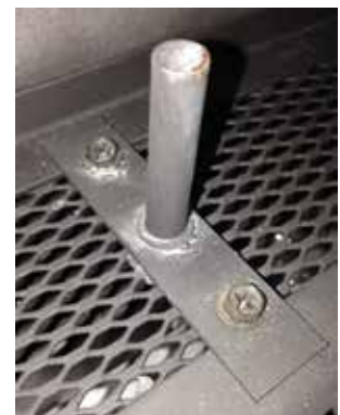
Figure 18 – Log Pin Assembly
