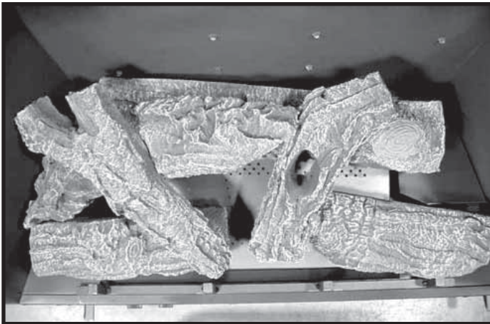
LOG #6 (SRV438-724): Position the "Y" end of log #6 into the cutout on log #4 and its opposite end into the groove on log #2.
