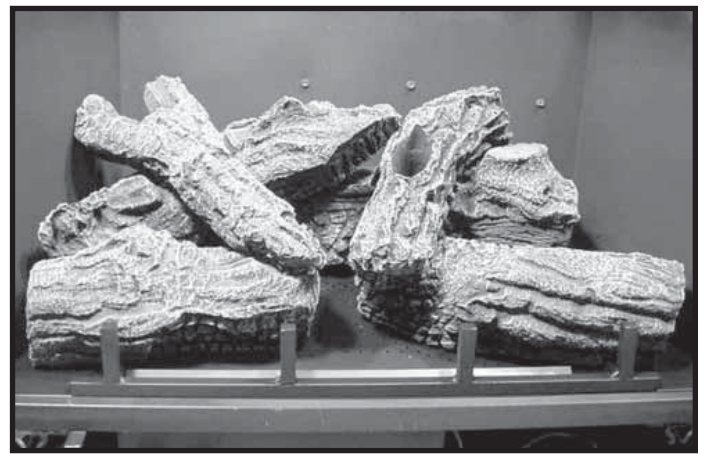
LOG #6 (SRV438-724): Position the "Y" end of log #6 into the cutout on log #4 and its opposite end into the groove on log #2.
