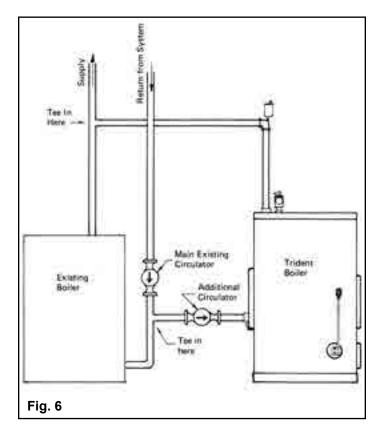
The circulator installed between the two boilers may be hooked up to run continuously during the heating season or, an additional S350 control (not supplied) could be installed to turn it on and off automatically. This control must be used as a "close on rise of temperature" (jumper in cooling position).
