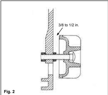
Bolt the Automatic Draft Control through the 1/2 in. hole in the center of the bottom door. Be sure to hold the Draft Control straight while tightening. Feed the two wires from the draft motor through the flexible conduit and a 90° fitting. Secure the fitting to the draft motor and that end of the conduit at this time. Check the flapper door on the Automatic Draft Control assuring that it moves freely.
