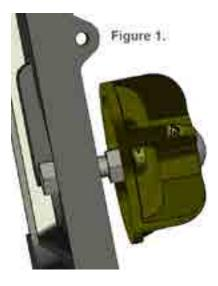
operation. **Warning:** Keep pieces of wood or coal out of the draft door opening mechanism, as this could cause the door to stick.
