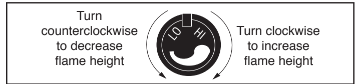
Figure 47 - Flame adjustment knob for Honeywell valve.
