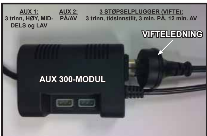
Figur 12.10 Plugg viften inn i AUX300CE-modulen
