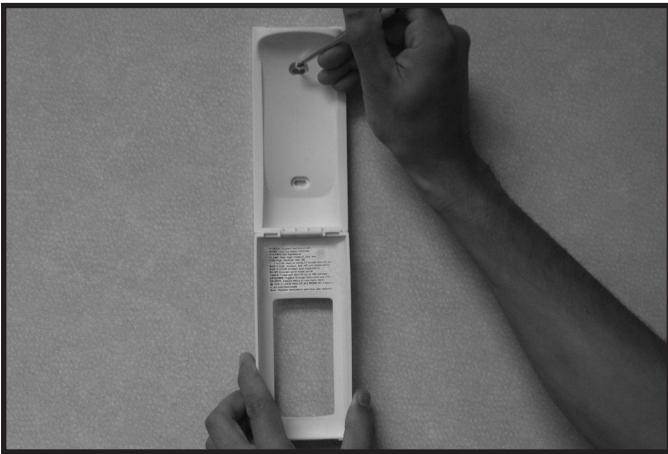
Figure 3.11 Mounting Remote Control Housing
