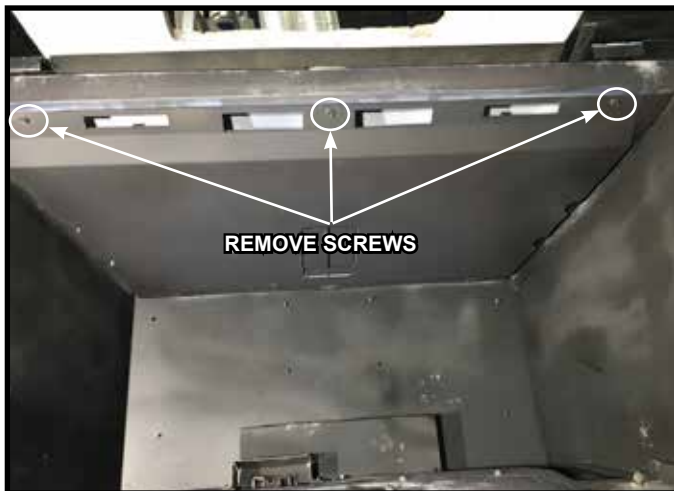
Figure 5.7 Remove Baffle Cover
