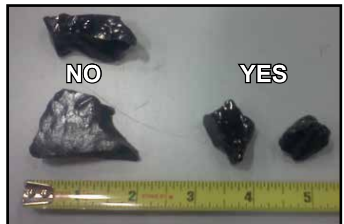
Figure 11.8 Selecting Flat Media for Pilot Cover.
