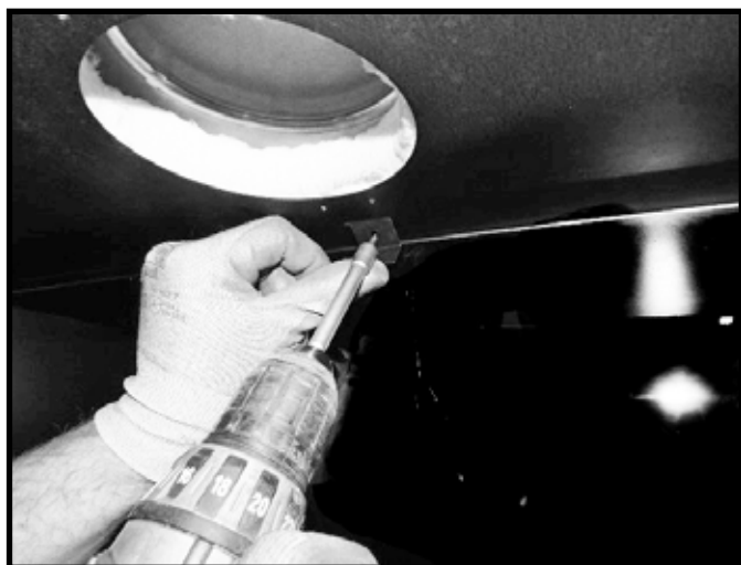
Figure 11.5 Install Back Glass Panel Retaining Bracket
