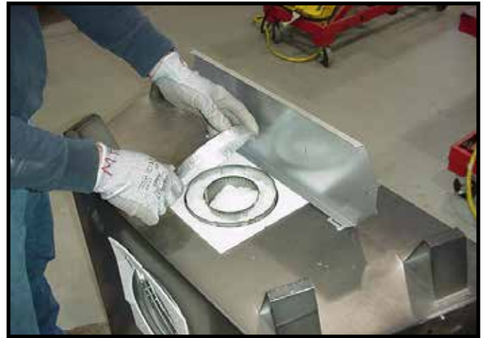
Figure 6.4 Remove the seal cap.
