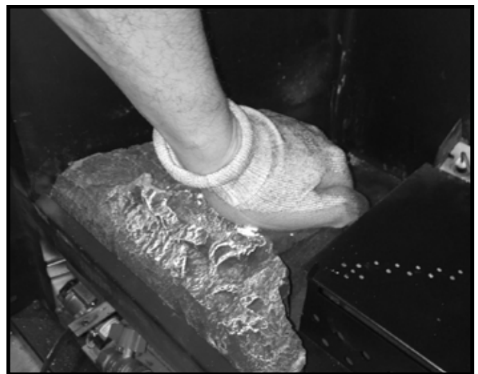
Figure 11.2 Press Left Hearth Firmly Into Place
