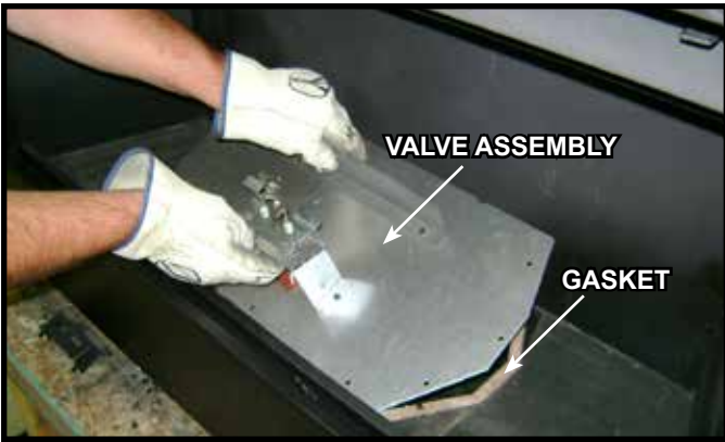
Figure 16.6 Remove Valve Plate
