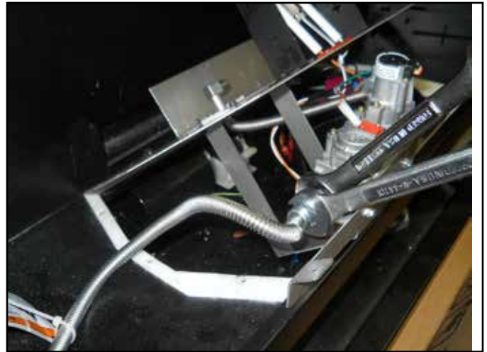
Figure 16.7 Disconnect Gas Valve
