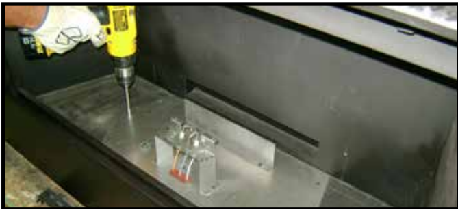
Figure 11.2. Remove Valve Plate Screws
