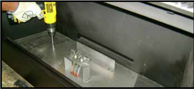
Figure 16.5 Remove Valve Plate Screws
