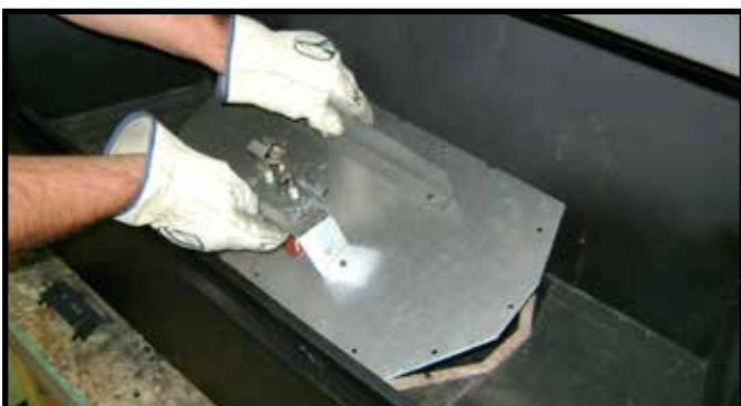
Figure 11.3. Remove Valve Plate
